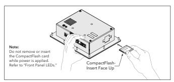
Information stored on a CompactFlash card by a PG6 can be read by a card reader attached to a PC. This information is stored in IBM (Windows®) PC compatible FAT16 file format.
