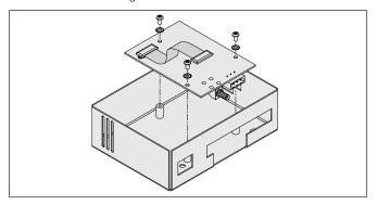
Connect the cable from the option card to CN11 on the main board of the PG operator interface as shown in Figure 3. Be sure both ends of the cables are firmly seated into their appropriate connector housing.
