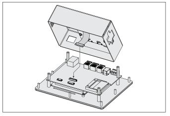
Carefully replace the rear cover by reversing the previous instructions for removing the rear cover. An external antenna must be attached to the bracket on the option card as shown below. See Antenna Connector in the Specifications section for more information.
