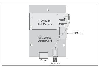
To install the option card remove all power and communication cables from the unit. The chassis ground connection to the rear cover may be left connected. The PG operator interface literature contains instructions for removing the rear cover, refer to the "Battery & Time Keeping" section.
