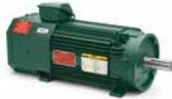
The RPM AC™ series of AC motors was designed specifically for optimum inverter duty performance, and offers high performance over a wide speed range. The compact, square cross-section, laminated steel frame includes cast iron brackets with feet for maximum ruggedness and stability. The unique low inertia design allows fast acceleration and high dynamic response. And to assure long and reliable motor life, Corona-Free insulation is used on all RPM ACTM ratings.
