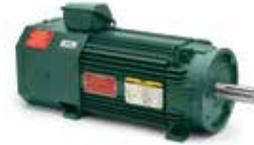
The RPM AC™ series of AC motors was designed specifically for inverter duty performance, and offers high performance over a wide speed range. The compact, square cross-section, laminated steel frame includes cast iron brackets with feet for maximum ruggedness and stability. The low inertia design allows fast acceleration and high dynamic response. And to assure long and reliable motor life, Corona-Free insulation is used on all ratings.
