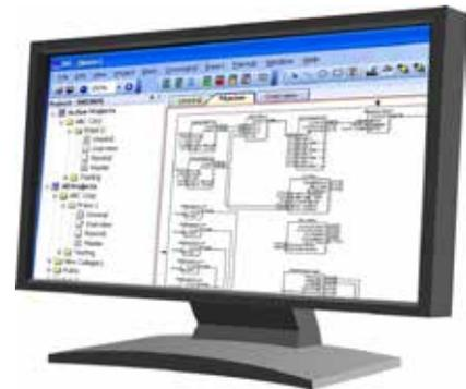
Using straightforward block programming, DSE allows the user to create, parameterize and configure user defined applications thanks to function blocks dedicated to speed control, inputs, outputs, ramps, winder functions, PID, diameter calculator, and more. Groups of function blocks can be combined into macros for more complex programs.
