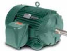
For applications in tougher environments, we offer V\*S Master™, featuring cast iron frame and end shields. Overload is no problem, with 200% capability for 60 seconds. Corona-Free insulation and an insulated CE bearing extend lifetime.
