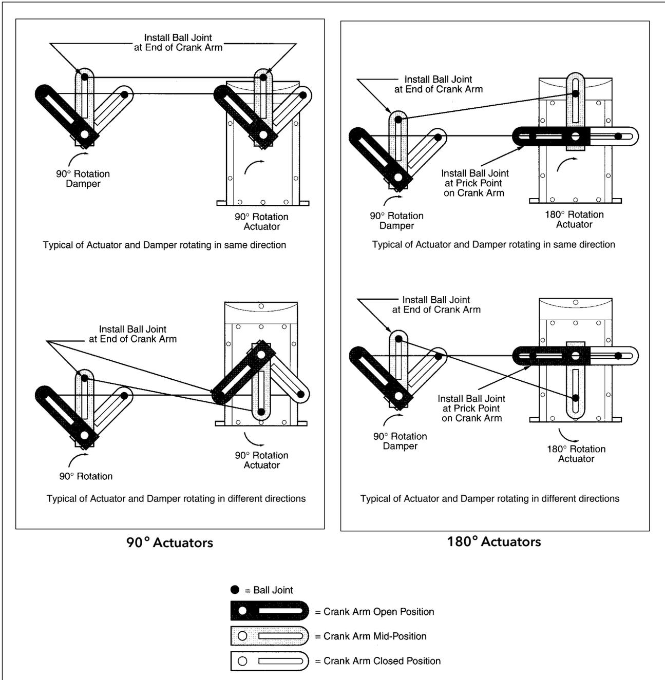
Figure 6. Typical Damper Linking
