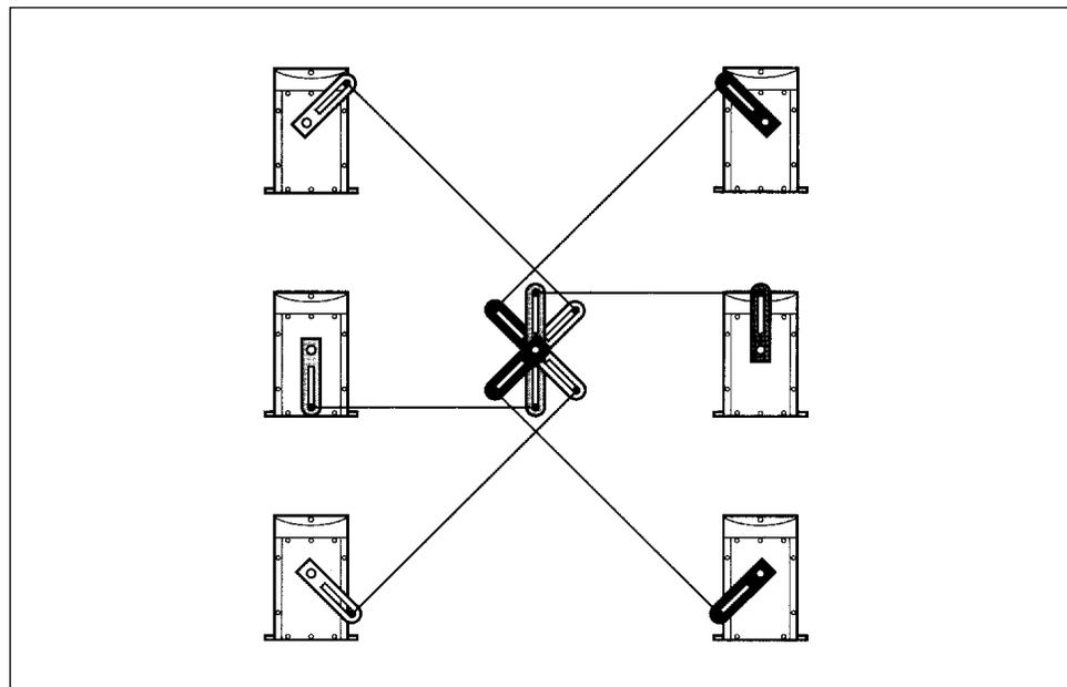
Figure 5. Typical Actuator Mounting Positions
