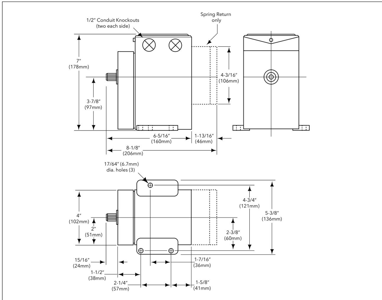
Figure 7. Mounting Dimensions, EA Actuator
