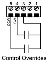
A dry contact closure between Terminal 3 and Terminal 4 will drive the actuator fully clockwise.
