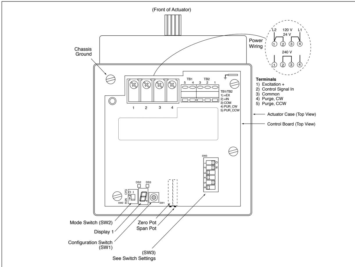
Figure 1. Controller board showing components used during setup and configuration
