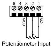
Input signals for potentiometers are connected to Terminals 1, 2 & 3. Terminal 1 is the CW connection; Terminal 2 is the wiper connection; Terminal 3 is the CCW connection.
