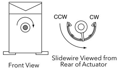
*Note the position of the slidewire as the shaft turns clockwise.*
