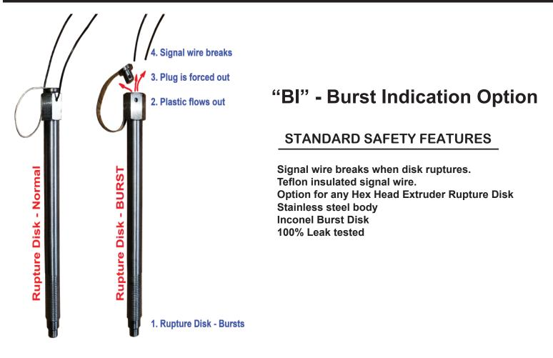
Extruder Rupture Disks with Burst Indication (option - BI) offers an inexpensive signal output when the disk ruptures. A plug is fitted at the discharge end. A small hole if drilled through the hex head where a small diameter teflon insulated signal wire is placed through. When a rupture disc discharges, plastic flow causes the plug to pop out and shear the signal wire. This sheared wire can be used to send a signal to the control system to shut the extruder down.
