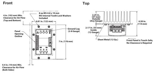
$<sup>^{\</sup>scriptsize\textcircled{1}}$  With the potential for high through-wall heat sink temperatures, application may require a touch-safe shield.
